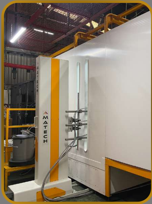
MATECH , PLC controlled Matech brand Paint center equipment; It is a complementary element of paint systems to improve paint quality and rapid color change.
